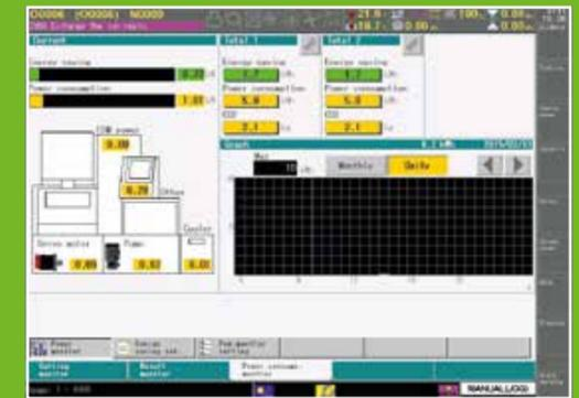
The energy saving function makes it possible to track precisely the amount of energy being consumed during machining or on standby. Power saving interventions such as switching off flushing or filter pumps can also be set, with features such as screen savers, sleep mode, auto start-up by timer and auto power off, all contributing to additional savings.
